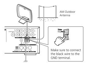
• If the AM loop antenna provided does not deliver sufficient reception (often due to being too far from the transmitter or in a concrete building, etc.), it may be necessary to use an outdoor AM antenna. Use either a high quality commercial AM antenna or, if not available, an insulated wire more than 5 m long, strip one end, and connect this to the terminal as shown.
